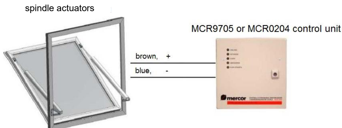
Fig. 17 Connection diagram for spindle actuators, without a lock.
