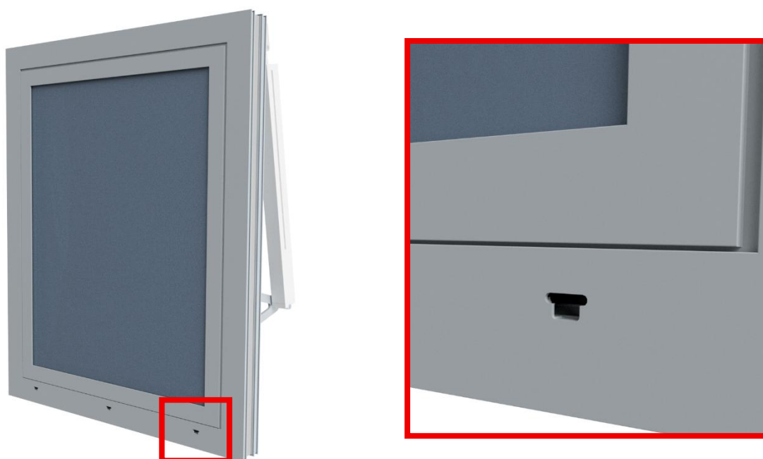
Fig. 13 Location and shape of drainage holes – inward-opening window.
